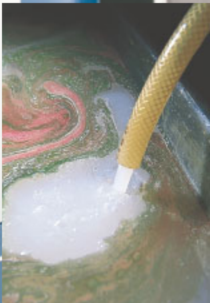
After cleaning, the coolant is returned to the tank.
