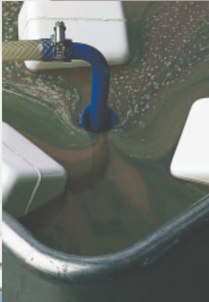
The contaminated coolant is skimmed from the surface.
